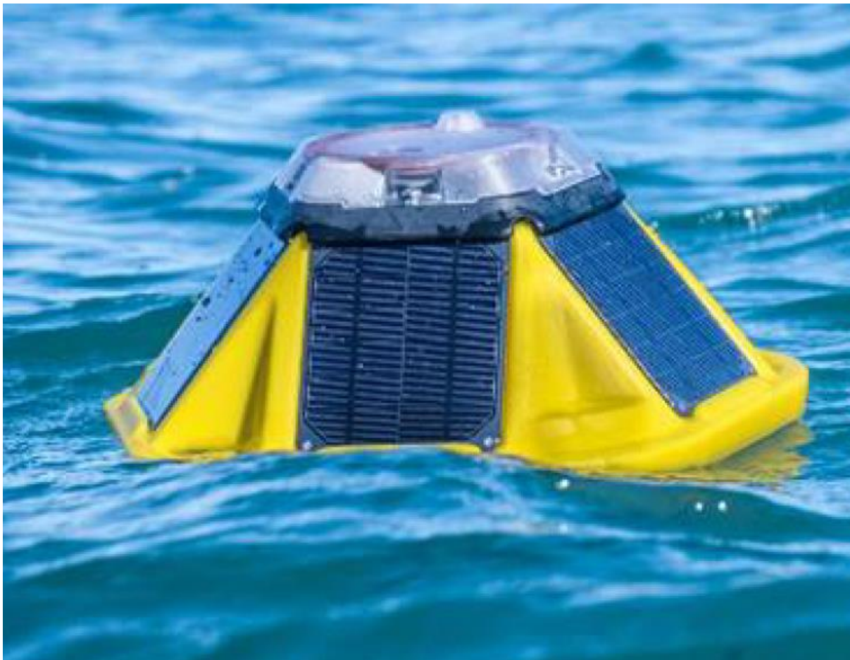
WAVE MONITORING BUOY
